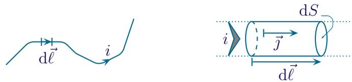
$$\begin{aligned} d\vec{f}_L &= d\mathcal{V} \vec{j} \wedge \vec{B} &= j \, dS \, d\ell \vec{T} \wedge \vec{B} \\ &= i \, d\vec{\ell} \wedge \vec{B} \end{aligned}$$
